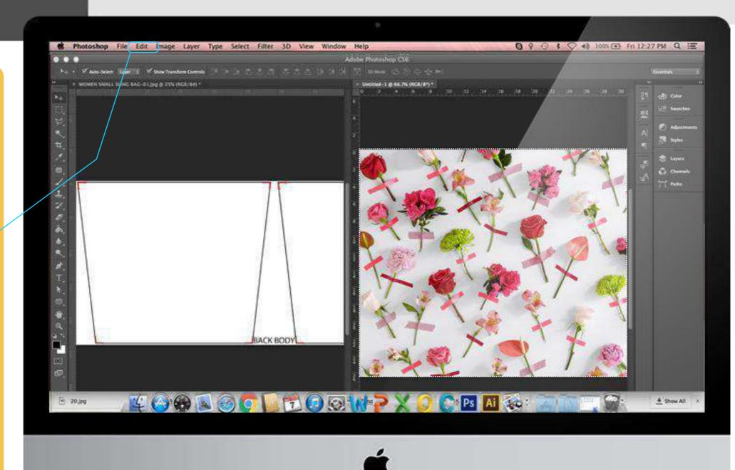
4. On the pattern file window, use the **Magic Wand** Tool (at tool bar on the left side) then left-click inside the part you want to work with
